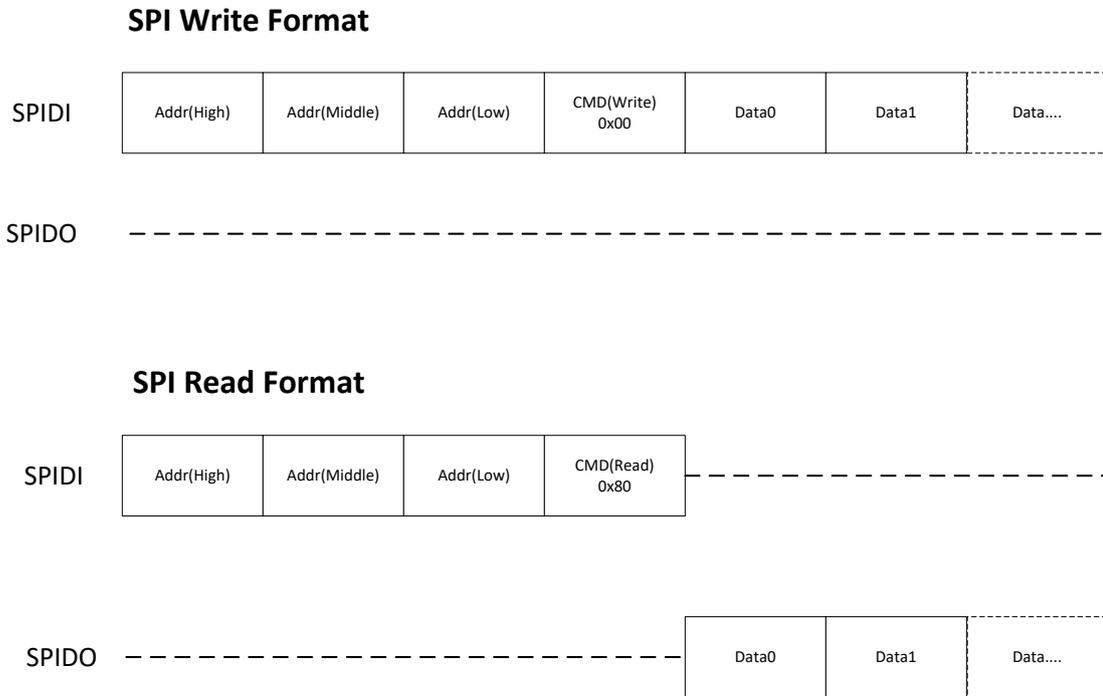
Figure 7-9 SPI write/read command format
