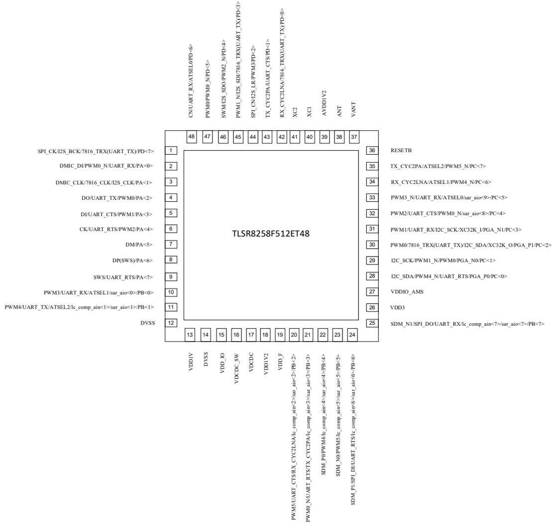
Figure 1- 4 Pin assignment for TSLR8258F512ET48
