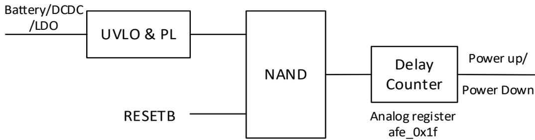
Figure 2- 3 Control logic for power up/down
