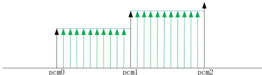
Figure 9-5 Delay interpolation
