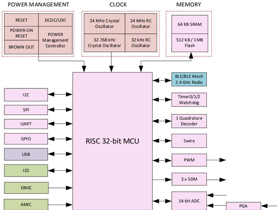
Figure 1- 1 Block diagram of the system
