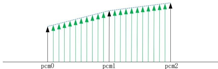
Figure 9-4 Linear interpolation
