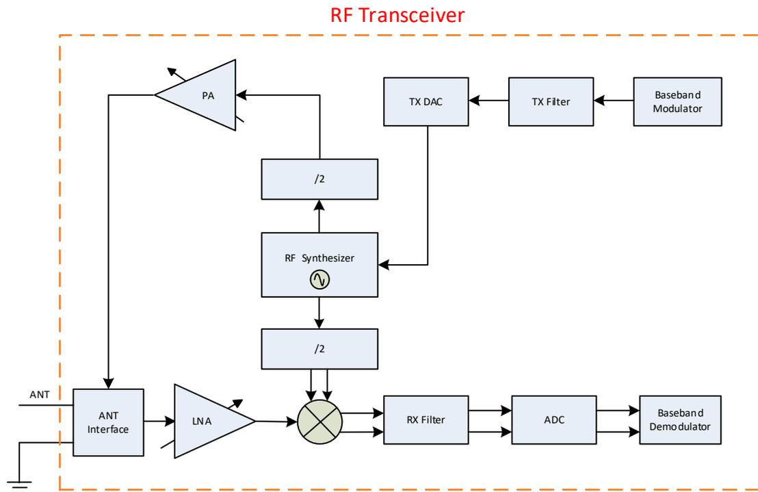
Figure 3- 1 Block diagram of RF transceiver
